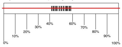
**Example:** If you have two bar codes next to one another and the centering window is set to 40% left edge and 60% right edge, only the bar code that intersects that window will be decoded.
